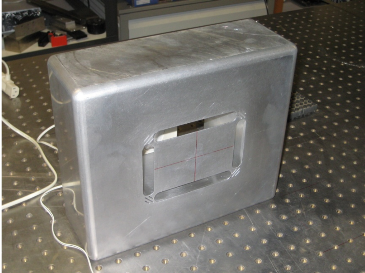
Fig. 1 Prototype of 'cyclic' Reference Material manufactured from cast aluminium alloy 5083 (Peraluman, AlMg4.5Mn0.7)
